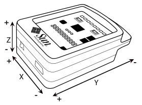
In FIGURE 8, the plus (+) on the end of an axis indicates that when the device's acceleration vector increases in that direction, the associated accelerometer readings will grow larger.
