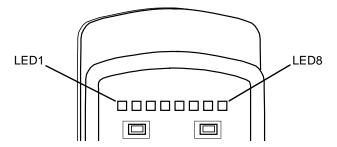
Each LED has a red, a green, and a blue emitter as part of the LED. Each individual color can have an intensity from 0 to 255, with 0 being off and 255 being as bright as possible.
