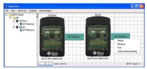
In the illustration, the SPOTs are both running the Bounce demo. The SPOT on the left is running in the main isolate, as shown by  $\mathbf{M}$  in the tree view. The SPOT on the right is running it as a child isolate.
